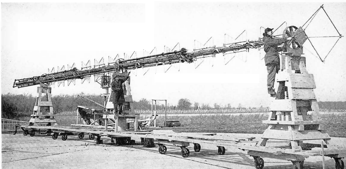
FIG. 9. In this view antenna was placed on a 12-foot high rotating mount and rotated about the electrical center during vertical pattern test.
