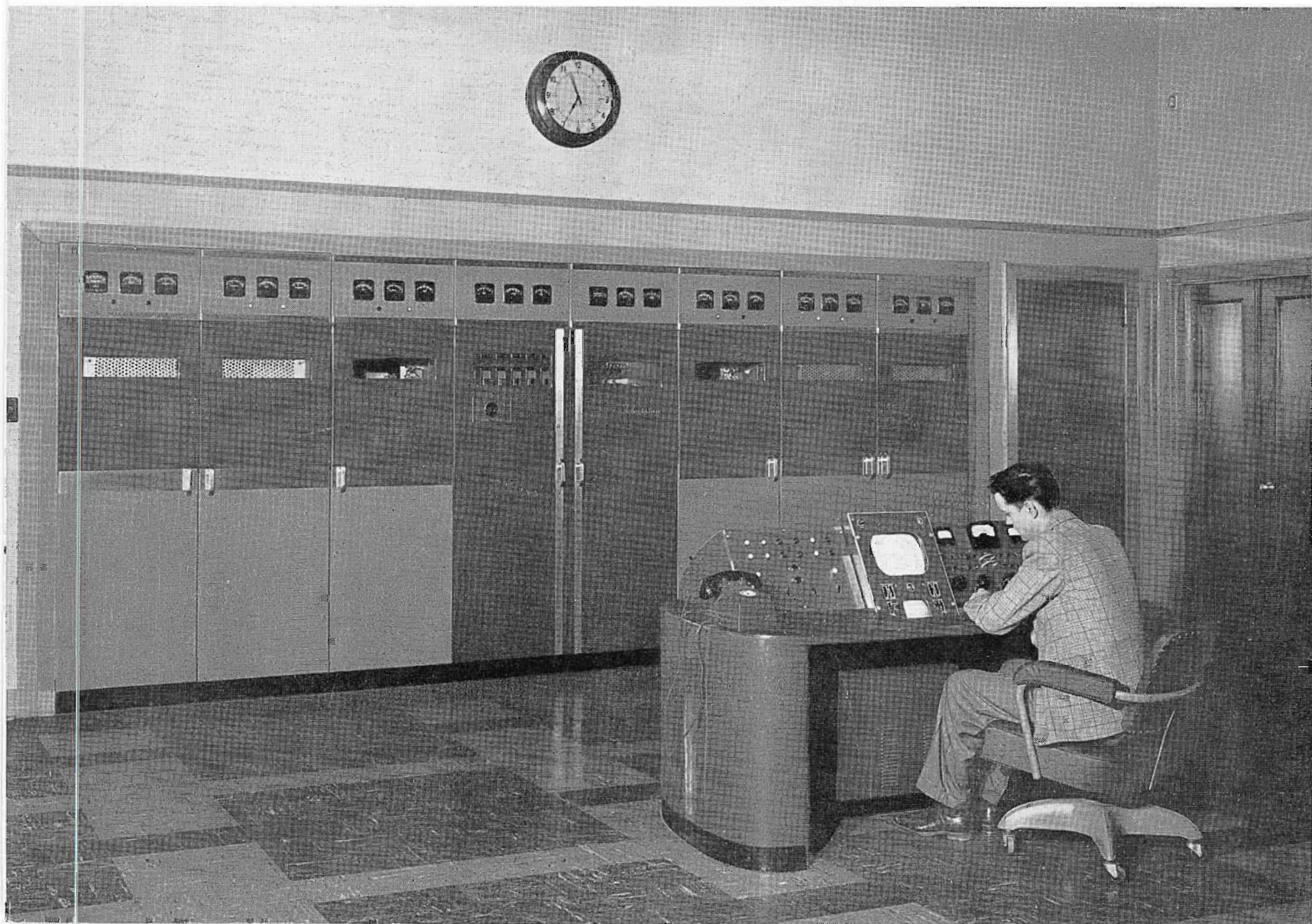
FIG. 8. CBFT Technician, Roland Berube, checking TT-5A Modulation. The test pattern can be seen as the picture was taken between the end of the Children's 5:00 to 5:30 P.M. Program and the start of the evening telecasts at 8:00 P.M.
